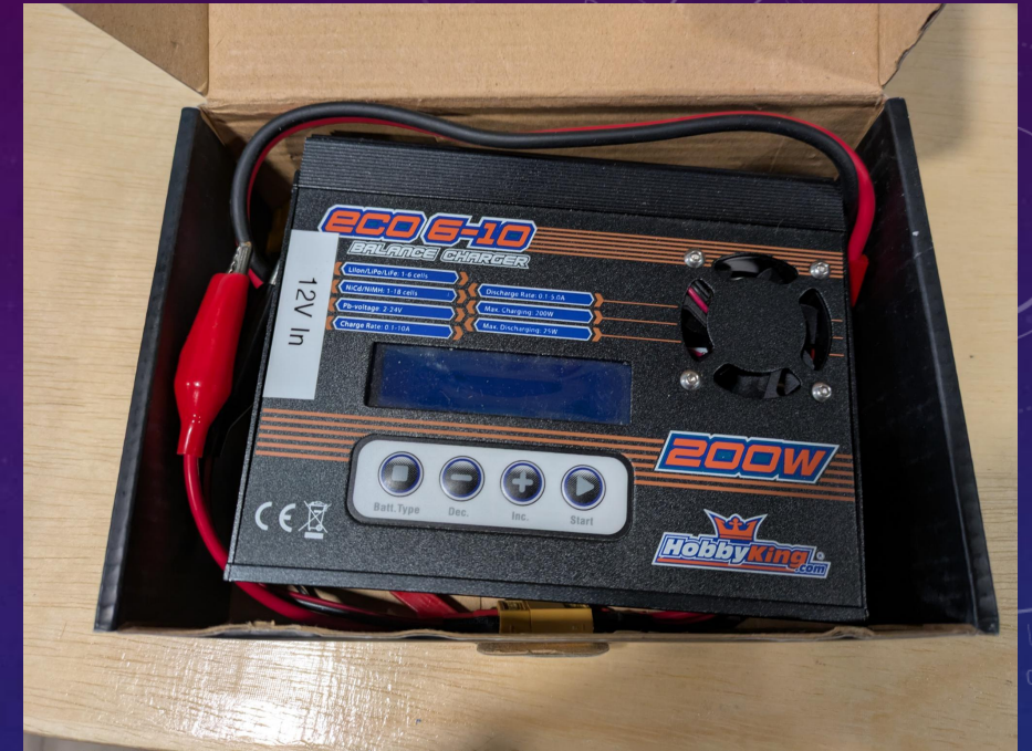
Cheap charger that supports multiple chemistries and battery voltages
